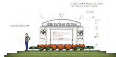
PYLON SIGN- FRONT ELEVATION SCALE: 1/4" = 1'- 0"
