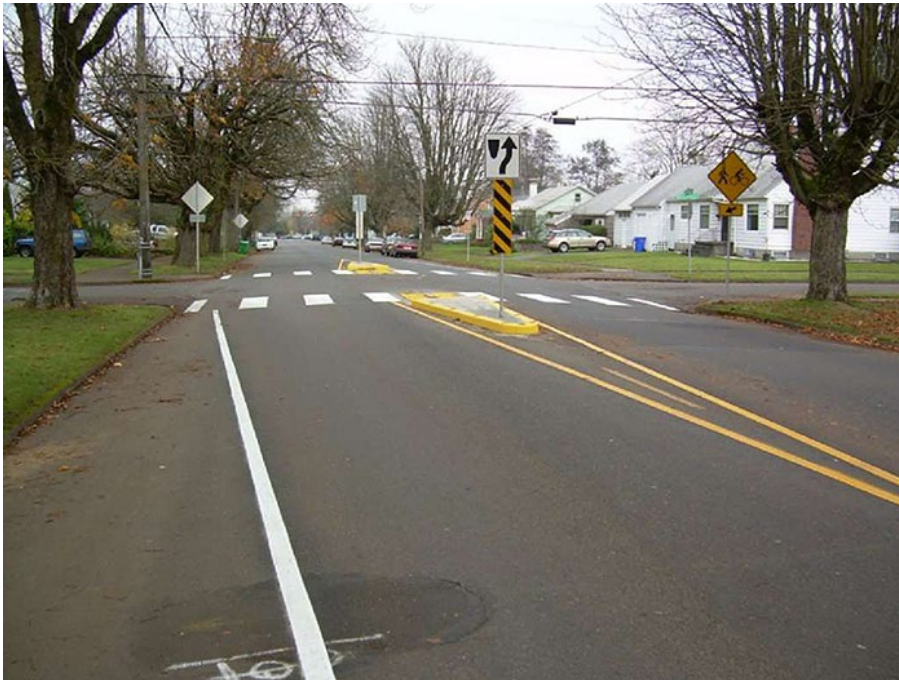
Figure 3.18.7. Small Median Islands at Intersection (Source: Scott Batson)
