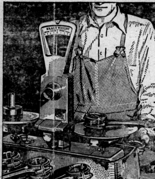
Chevrolet connecting rods are matched in sets of six to within one-quarter ounce, and are individually fitted by hand to the crankshaft. Bearings are of Babbitt metal cast into the rods under heavy air pressure and at 800 degrees Fahrenheit.
