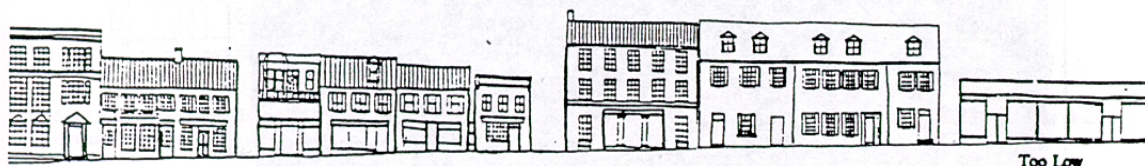
Lack of rhythm in building height occurs after the construction of a one-story building on the corner of a block (shown far right)
