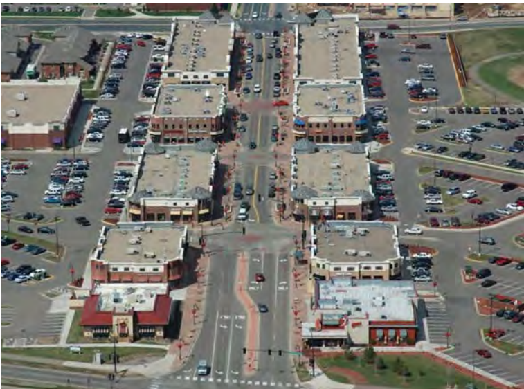
Surface parking areas located at rear of buildings fronting active street corridors.
