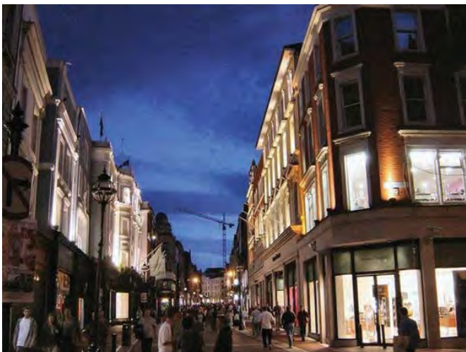
Building lighting providing indirect lighting for pedestrian areas.
